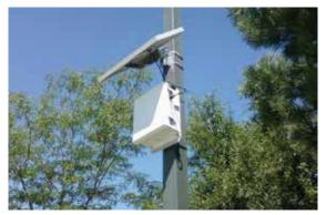
Figure 12: Photo. Example of a bluetooth antenna installation. (Source: JUB Engineers, Inc.)
