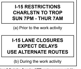
Figure 7. Illustration. Examples of CMS warning messages posted by FAST personnel for work activity on I-15. (Source: G.C. Wallace, Inc.)
