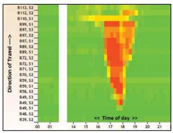
Figure 9. Chart. Example of a speed contour map generated using FAST data. (Source: FAST)
