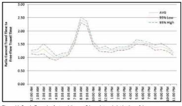
Figure 14: Graph. Example of a travel time confidence interval plot by time of day. (Source: JUB Engineers, Inc.)
